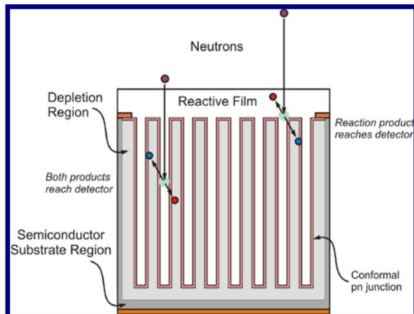
Fig. 2. The deep microstructures backfilled with neutron reactive material increase *both* neutron absorption efficiency and the reaction production detection efficiency for MSND<sup>®</sup>s.
