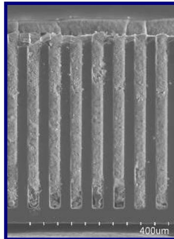
Fig. 3. MSND® side profile showing 490 micron deep microstructures backfilled with compacted  $^6\text{LiF}$ .
