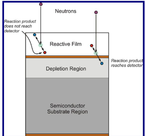
Fig. 1. For a coated planar detector, reaction product self-absorption limits film thickness, and consequently the detection efficiency.
