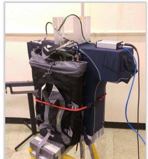
Figure Above: Li-Foil MWPC Backpack V1.0 (w/o the gamma-ray component) calibrated on an acrylic phantom.
